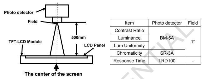
Note 2: Definition of viewing angle range and measurement system.
